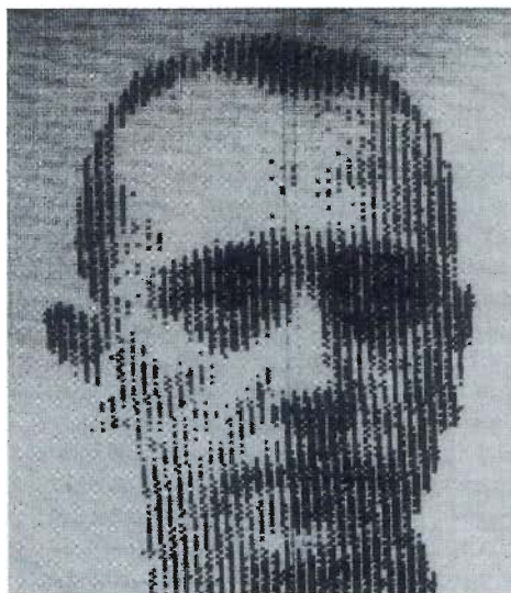
1.3 One of the first digital images: this picture was scanned from a photograph by the NBS mechanical drum scanner, processed by the SEAC computer, and displayed on an oscilloscope.
