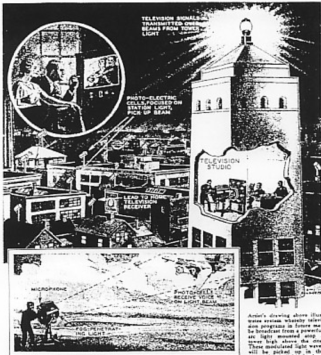
Airport supervisor directs plane landing over voice-modulated beam of light. Photo-cells on plane pick up beam, which is transformed back into voice speaking directions.
